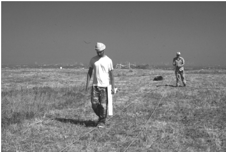
Figure 5.2. Magnetic field gradient survey at LAN-63 using the FM 36 fluxgate gradiometer.
