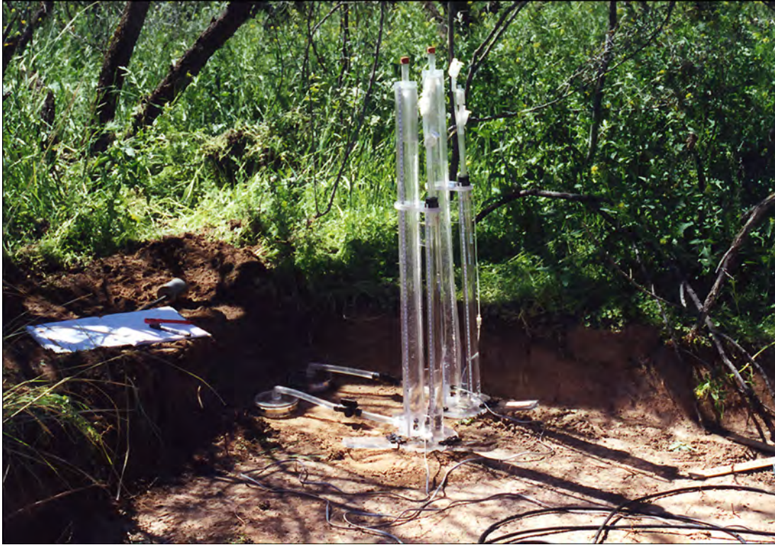
Figure 18. Photograph of tension infiltrometers testing the 25-cm-depth level of Trench 2.
