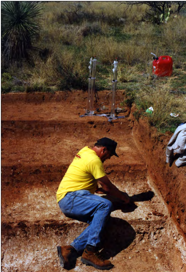
Figure 18. Photograph of tension infiltrometers testing the 25-cm-depth level of Trench 2.
